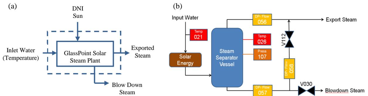
Figure 5: (a) Test boundaries, (b) Simplified schematic
